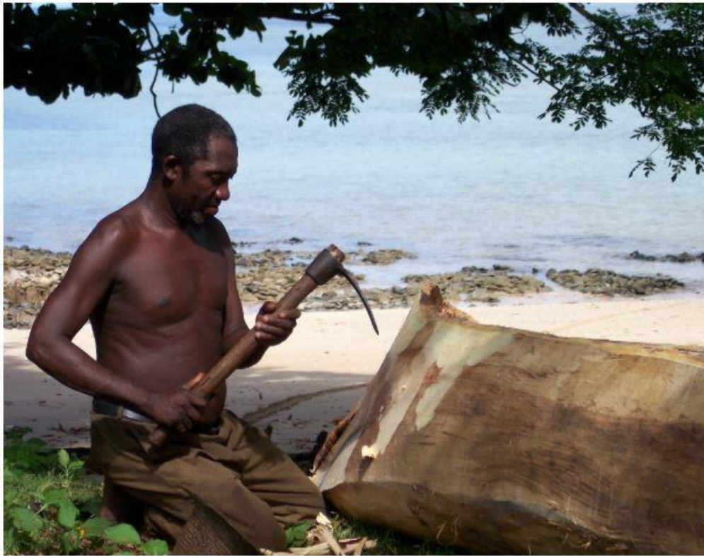
The main body of a pirogue being fashioned from a msiro ( Albizia saman ) tree – one of the ideal species for the purpose. (Credit Richard Davies 9 )
