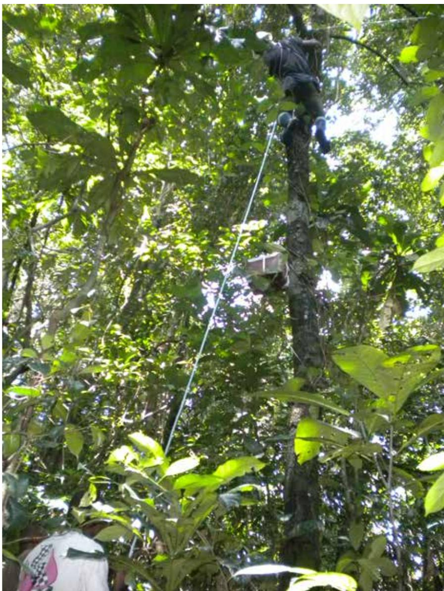
Lifting ARU 8m into tree to increase the sensor's detection range of gunshots, Credit: WildCRU
