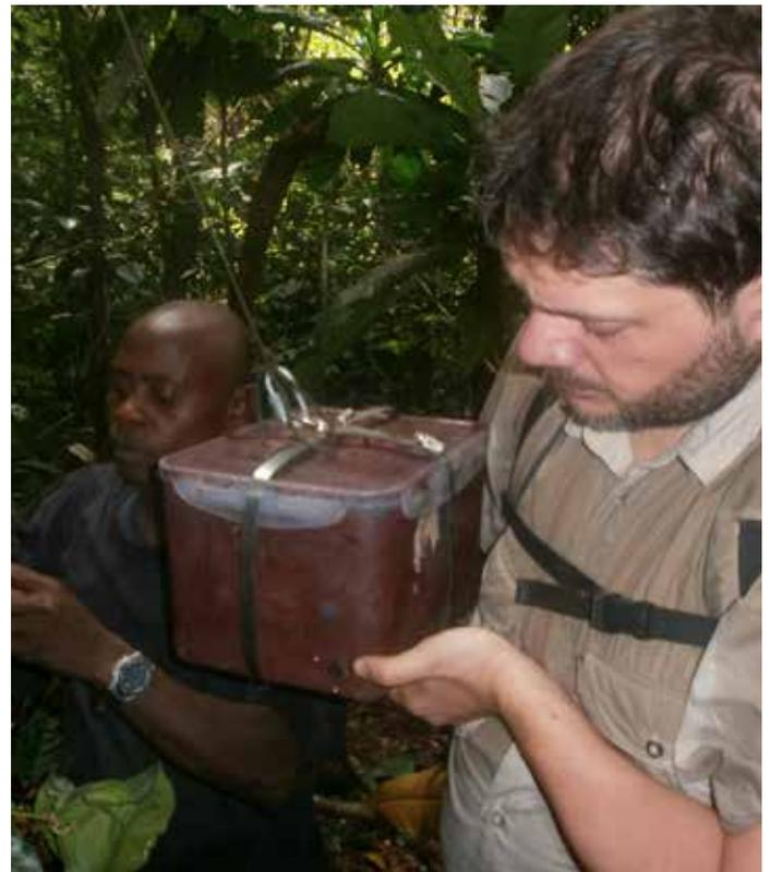
Setting up one of the Autonomous Recording Units (ARUs) used to monitor gunshots, Credit: WildCRU
